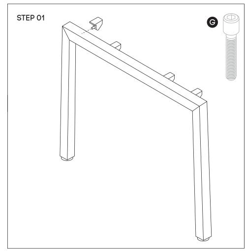
Using Allen Key provided, attach 4 plastic brackets per leg **(D)** (as per picture above) using M6x20MM **(G)** Socket head screw.
