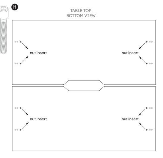
Place desktops ontop of frame - with cutout at the back of the desk. Nut inserts in top will align with plastic joiner brackets using M6x30MM **(H)** sockets attached tops to frame.
