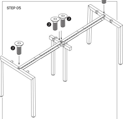
Attach beam **(F)** to legs **(C)** and Connector frame **(E)** using nut insert in legs. See point attached
