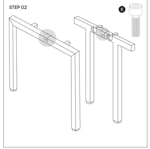
Using Allen Key provided, attach M8x20MM Socket head **(K)**-screw socket half way into leg for both legs **(C)** and into Connector frame **(E)**.
