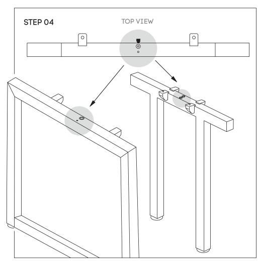
Attach beam **(E)** to legs **(B)** and Connector frame **(D)** using nut insert in legs. See point attached
