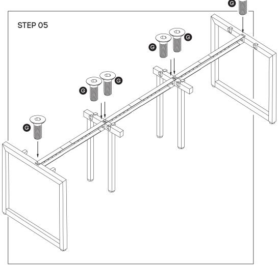
Frame looks like this. Using Allen Key, attach beam (E) with Socket (G)
