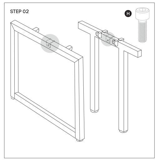
Using Allen Key provided, attach M8x20MM Socket head **(H)**-screw socket half way into leg for both legs **(B)** and into Connector frame **(D)**.
