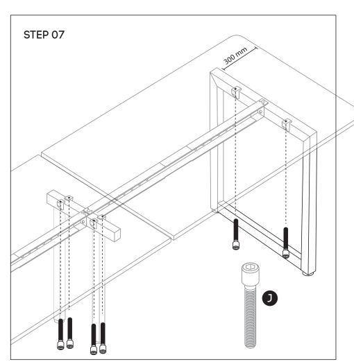
Please tighten M6x30MM Socket head (1) through the plastic brackets into the underneath of the tops.
