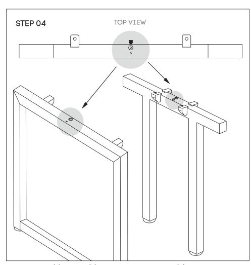
Attach beam **(E)** to legs **(B)** and Connector frame **(D)** using nut insert in legs. See point attached
