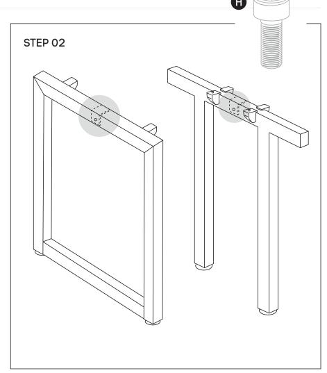
Using Allen Key provided, attach M8x20MM Socket head **(H)**-screw socket half way into leg for both legs **(B)** and into Connector frame **(D)**.
