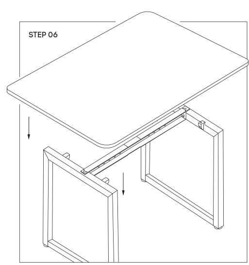
Place the desktop on top of the frame. Please place the legs ideally indented around 300mm from each end left and right of the Tops, Place the legs centred at the same distance equally from the front and back of the top.
