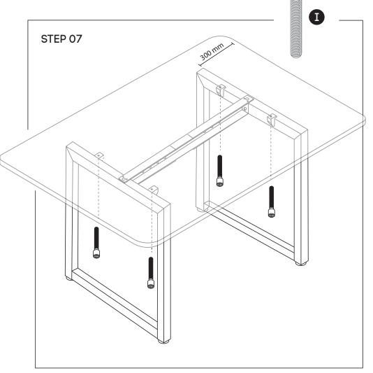
Please drill M6x30MM Socket head (I) through the plastic brackets into the underneath of the tops.
