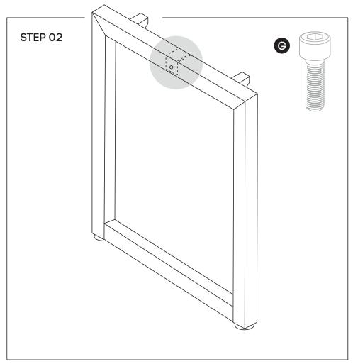
Using Allen Key provided, attach M8x20MM Socket head (G)-screw socket half way into leg for both legs (B)
