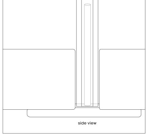
Second person to drill 4 holes into the brackets holes with provided wood screws into the underneath desktop. Please check the position of the rod brackets and bracket holes again before drilling the screws all the way through. Please tighten all the wood screws.
