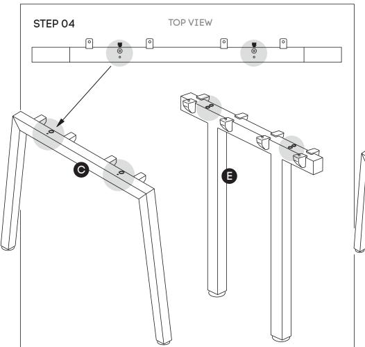
Attach main desk beams **(F)** to legs **(C)** and Connector frame **(E)** using nut insert in legs. See point attached
