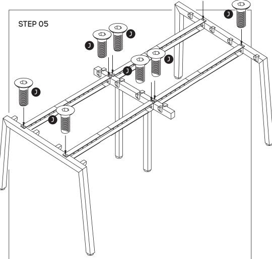
Frame looks like this. Using Allen Key, attach main desks beams **(F)** with Socket **(J)**
