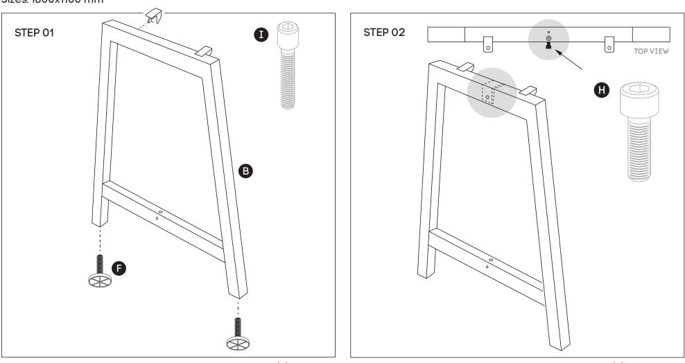
Using Allen Key provided, attach 2 plastic brackets per leg **(D)** (as per picture above) using M6x20MM **(I)** Socket head screw. Screw the feets **(F)** to the bottom of each leg **(B)**  Using Allen Key provided, attach M8x20MM Socket head **(H)**screw socket half way into leg for both legs **(B)**
