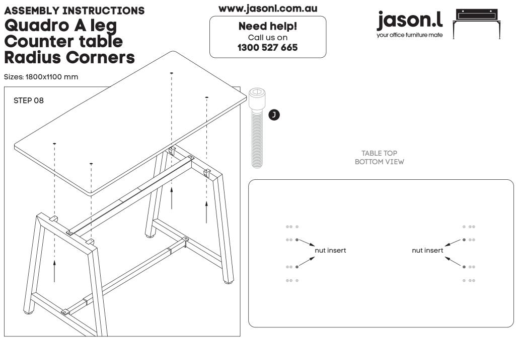
Place desktop on top of frame. Please tighten screws using M6x30MM (J) into the underneath of the tops.
