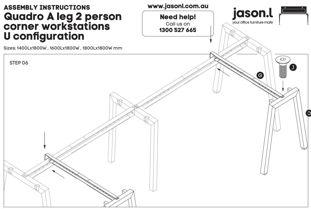
Now attach the return beams **(G)** to return legs **(D)** using nut insert in legs. See point attached. Then, connect the hook of the return beam to the beam of the main structure.
