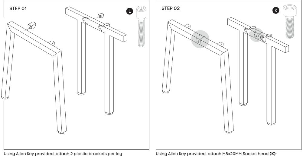
Using Allen Key provided, attach 2 plastic brackets per leg (C)(D) (as per picture above) using M6x20MM (L) Socket head screw. Do the same with Connector frame (E).
