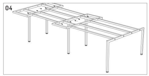
Add both connector frames together appropriate beams (4x1400mm).
