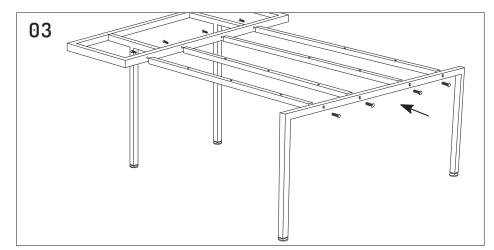
Attach 4x 1400mm beams to 1625mm leg using M8x25mm dome head screw. Attach connector frame from diagram 2 to 4 beams using M8x25mm dome head screws.
