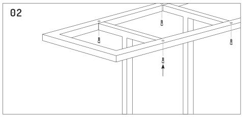
Assemble connector frames. Attach the 2 T legs to the double connector frame using M6x35mm hex scews x4.
