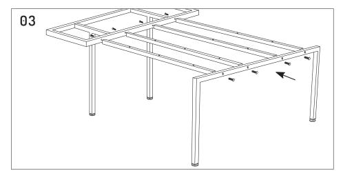
Attach 4x 1600mm beams to 1625mm leg using M8x25mm dome head screw. Attach connector frame from diagram 2 to 4 beams using M8x25mm dome head screws.
