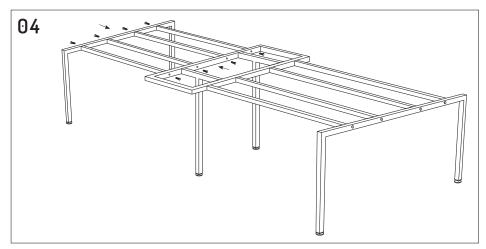
Attach the remaining 4x 1600mm beams to the connector frame using M8x25mm dome head screw.
