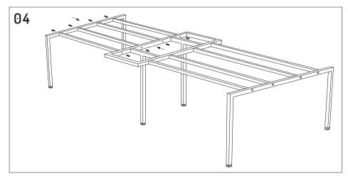
Attach the remaining 4x 800mm beams to the connector frame using M8x25mm dome head screw.
