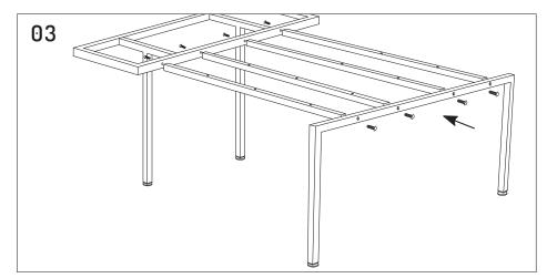
Attach 4x 800mm beams to 1625mm leg using M8x25mm dome head screw. Attach connector frame from diagram 2 to 4 beams using M8x25mm dome head screws.
