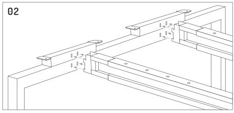
Use the two beams to connect the legs.
