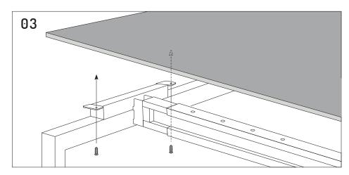
Attach legs + beams to Desks Top by tightening Screws.
