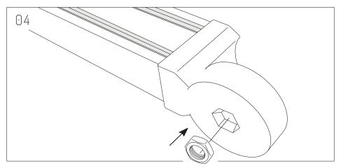
Insert Hex Nut on each Beam Bracket.
