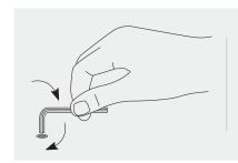
If this bolt does not drop into the joint use the Allen key to screw it all the way in so that it creates its own thread.
