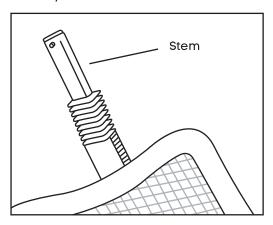
**STEP 5**Push stem through the hole to the desired height.
