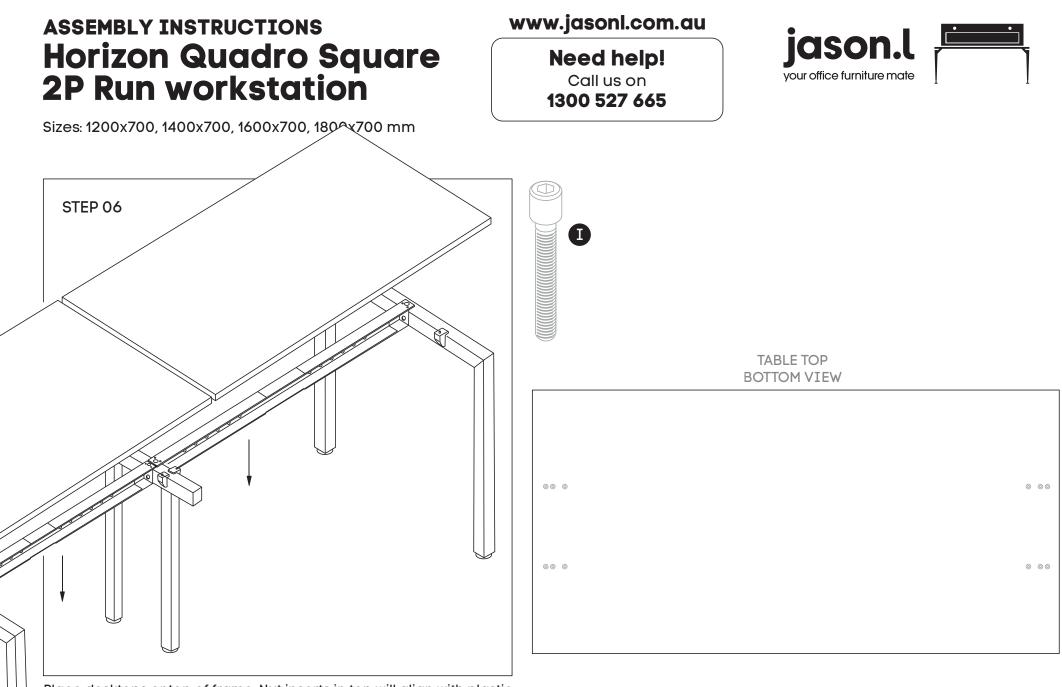
Place desktops ontop of frame. Nut inserts in top will align with plastic joiner brackets using M6x30MM **(I)** sockets attach tops to frame.
