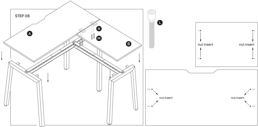
Place table top (A) ontop of frame - with cutout at the back of the desk. Using nut inserts in the desk, use M6x30mm socket (L) and attach desktop to the frame.
