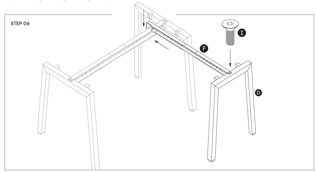
Now attach the return beam **(F)** to return leg **(D)** using nut insert in legs. See point attached. Then, connect the hook of the return beam to the beam of the main structure.
