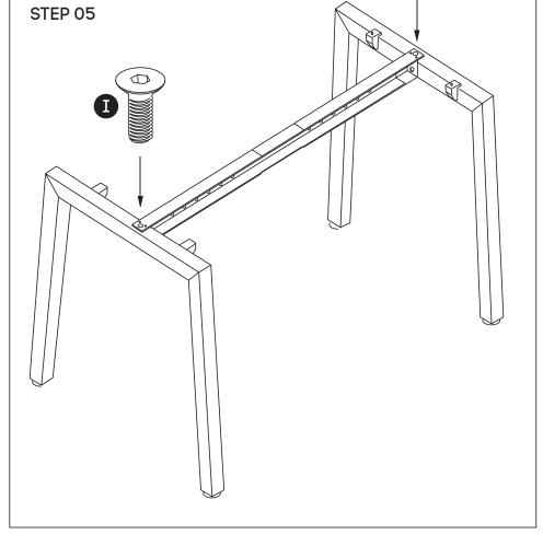
Attach beam **(E)** to legs **(C)** using nut insert in legs. See point attached
