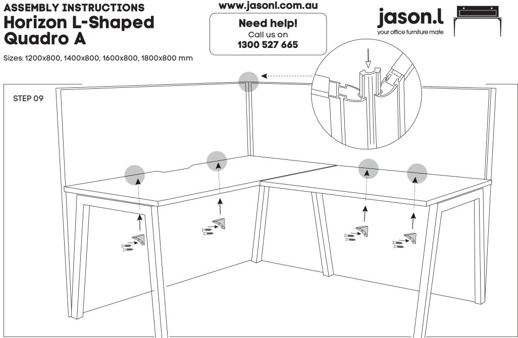
Using an Allen Key remove the top 2 caps from screens uprights. Bring two partition towards one another and slide the 90 degree connector rod - down between the two screen uprights. Under the desktop, use 4 I-shaped panel brackets to secure the screens to the desktops.
