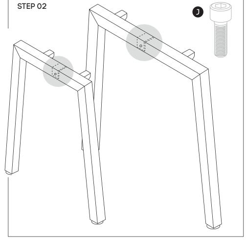
Using Allen Key provided, attach 2 plastic brackets (G) per legs (C & D) (as per picture above) using M6x20MM (K) Socket head screw.
