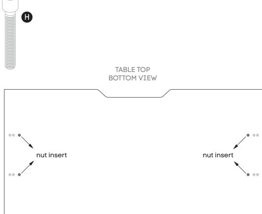
Place desktop ontop of frame - with cutout at the back of the desk. Nut inserts in top will align with plastic joiner brackets using M6x30MM **(H)** sockets attached top to frame.
