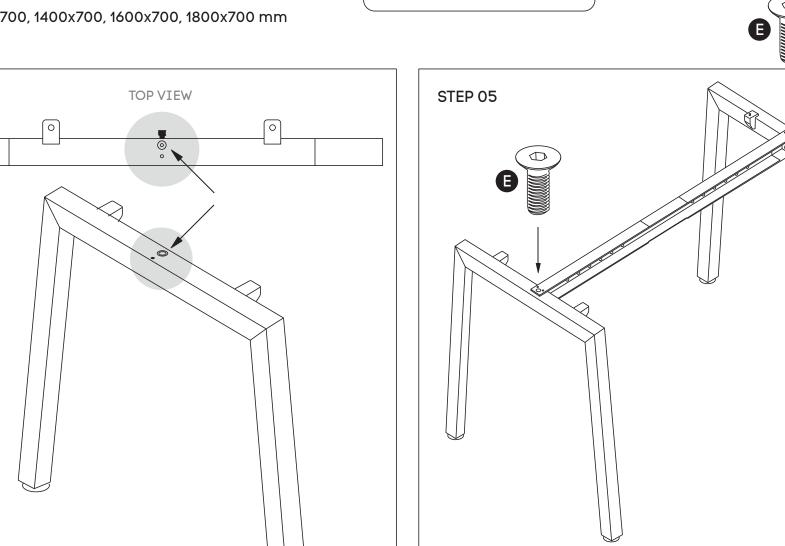
Attach beam (C) to legs (B) using nut insert in legs. See point attached
