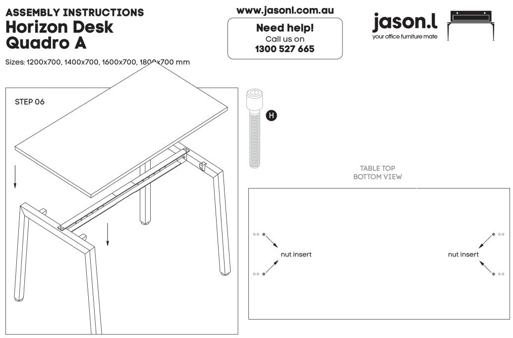
Place desktop ontop of frame. Nut inserts in top will align with plastic joiner brackets using M6x30MM **(H)** sockets attach top to frame.
