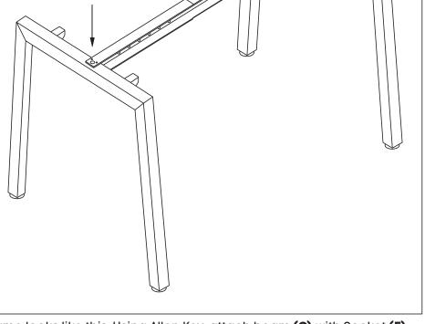
Frame looks like this. Using Allen Key, attach beam (C) with Socket (E)
