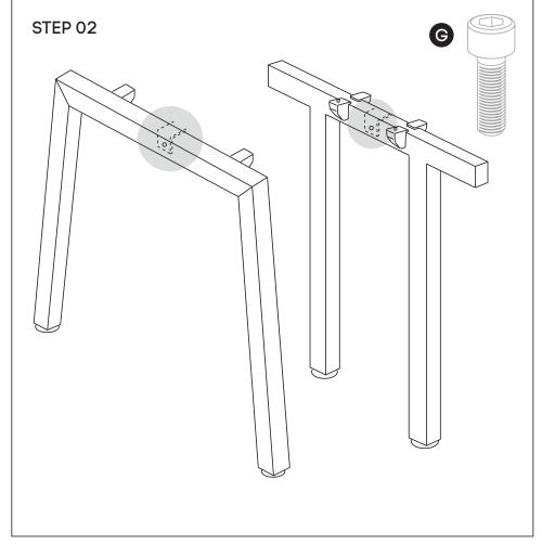
Using Allen Key provided, attach M8x20MM Socket head (G)-screw socket half way into leg for all legs (B) and into Connector frame (C).
