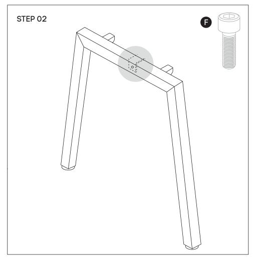
Using Allen Key provided, attach M8x20MM Socket head (F)-screw socket half way into leg for all legs (B).
