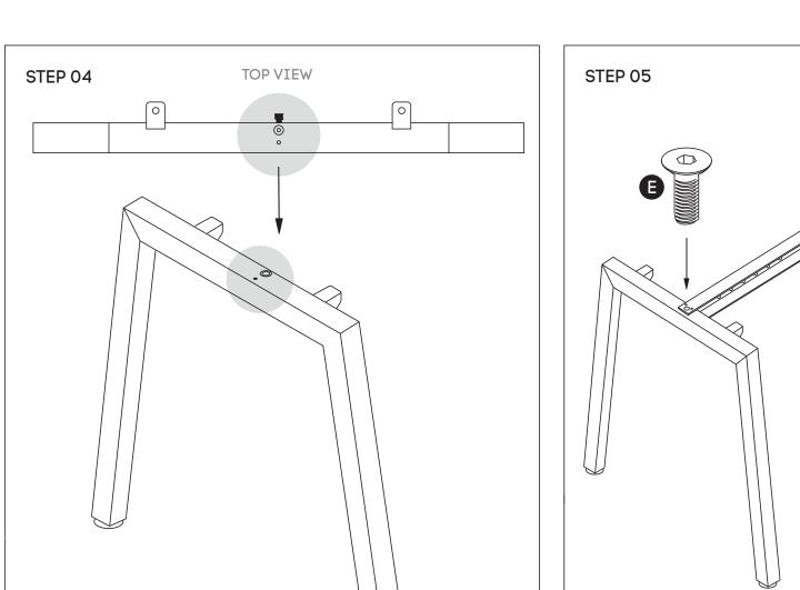
Attach beam **(C)** to legs **(B)** using nut insert in legs. See point attached
