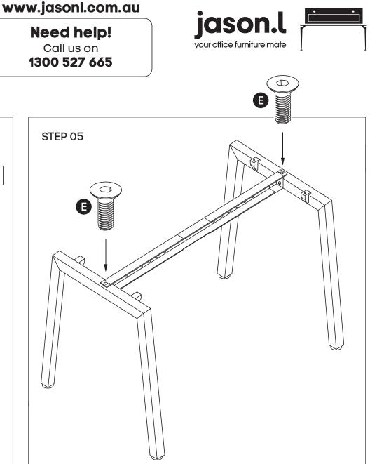
Frame looks like this. Using Allen Key, attach beam (C) with Socket (E)
