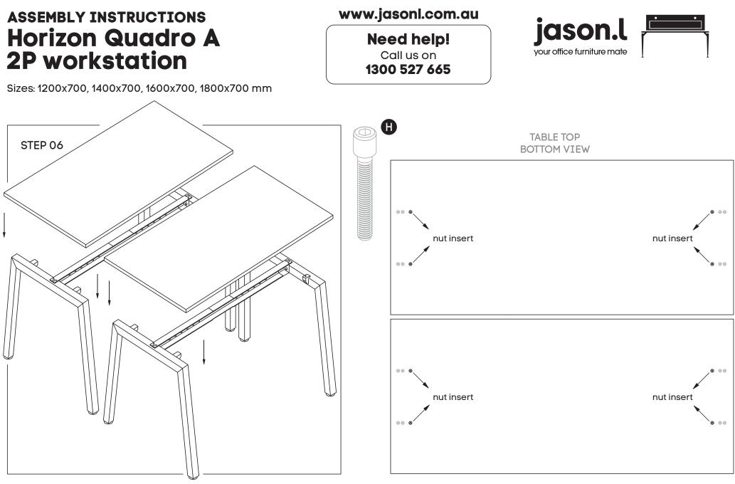
Place desktops ontop of frame. Nut inserts in top will align with plastic joiner brackets using M6x30MM **(H)** sockets attach tops to frame.
