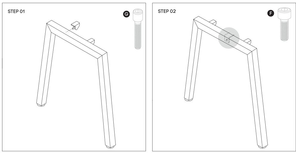
Using Allen Key provided, attach 2 plastic brackets per leg **(D)** (as per picture above) using M6x20MM **(G)** Socket head screw. Using Allen Key provided, attach M8x20MM Socket head (F)screw socket half way into leg for all legs (B).
