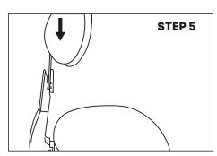
Insert the stem firmly into mechanism at the back bottoms out. Therachet height adjustor works like a car head rest. Press all the way down then lift to required position. When back is in place, remove elastic band.
