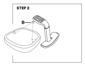
Tip chair seat upside down. Rest seat on corner of a table. Attach arm to chair seat using B spacer on the one hole each left and right arm.
