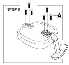
Attach arm using 6 x M6\*35mm (3 on the left armand 3 on the right arm). Tighten screws all the way down into the chair seat.
