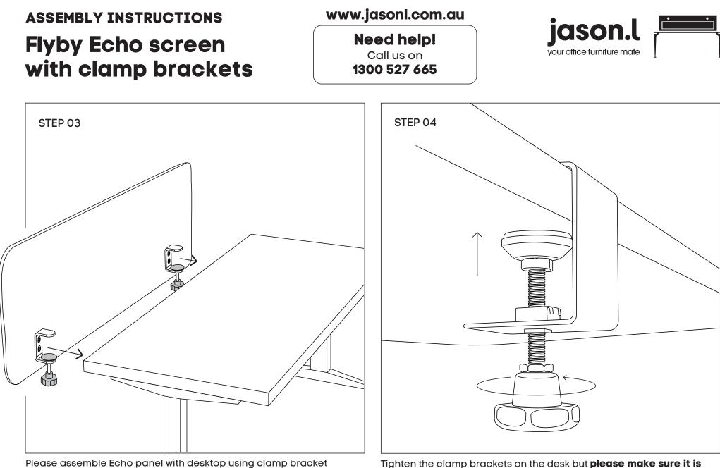
Tighten the clamp brackets on the desk but **please make sure it is still a bit loose** so that you are still able to move around the screen to its final position on desk and then **tighten the knob**.
