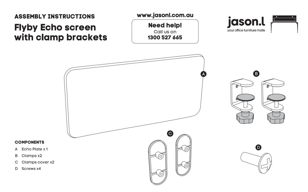
Experienced assembly is required. User will need to drill wood screws into underside of desk. No pre-drilled holes are provided for this system.
