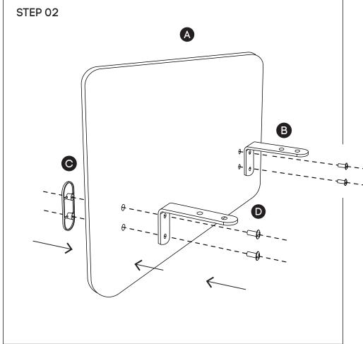
Assembe A plate with B bracket and tighten using 4 x screws provided (D) and apply the bracket cover C
