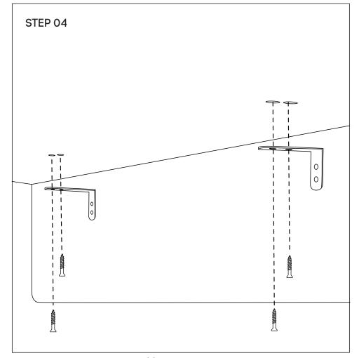
Please drill 4 x wood screws (**E**) into the underneath desk and tighten the L brackets on the desk.
