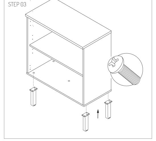
Attached plate to leg, using 2 flat head screws
