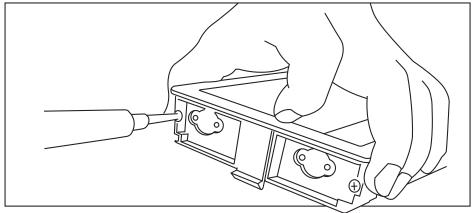
You will see two screws on the sides as illustrated in the image. Unscrew them to remove the side cover. Once you have done this on both sides, you will be able to slide the components out.
