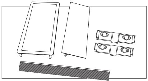
Diagram of the product completely disassembled. To reassemble, simply slide the parts back inside, place both side covers to secure all the pieces, and finally screw them in place.
