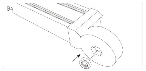
Insert Hex Nut on each Beam Bracket.
