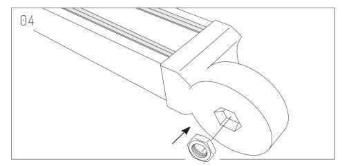
Insert Hex Nut on each Beam Bracket.
