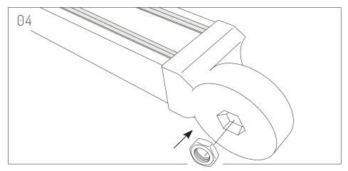
Insert Hex Nut on each Beam Bracket.
