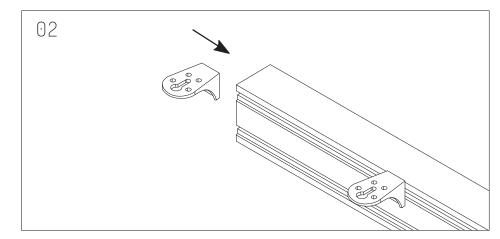
Join 2 L-Bracket through each 625mm Beam and 1 L-Bracket through each 1315mm Beam
