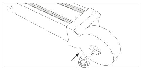
Insert Hex Nut on each Beam Bracket.
