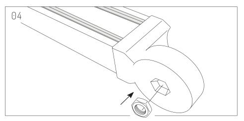
Insert Hex Nut on each Beam Bracket.
