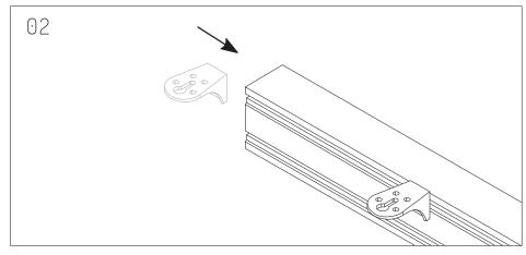
Join 1 L-Bracket through each Beam.
