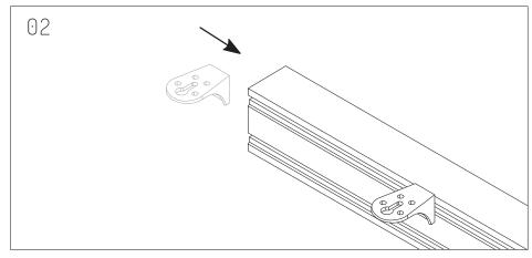
Join 1 L-Bracket through each Beam.
