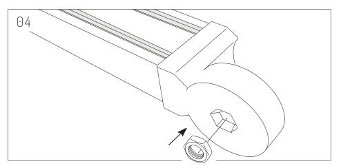
Insert Hex Nut on each Beam Bracket.
