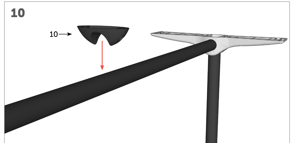
Locate the plastic support bracket 10 over the centre of both top rails, and click into place.
