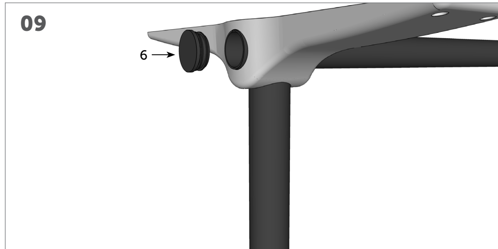
Place the top rail cap 6 into the exposed end of the top rails.
