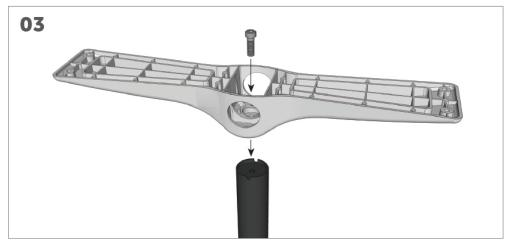
Place the upper wrist on top of the leg tube, making sure each small notch in the top of the leg tube is in-line with the bumps on the bottom of the upper wrist. Fully tighten to maximum tension the M10x30mm bolts.
