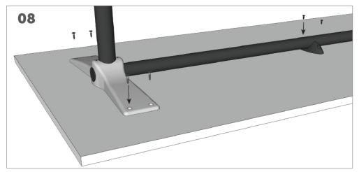
With the frame assembly complete, locate it in the centre of the work surface and screw the remaining self tapping screws into each upper wrist and plastic support.
