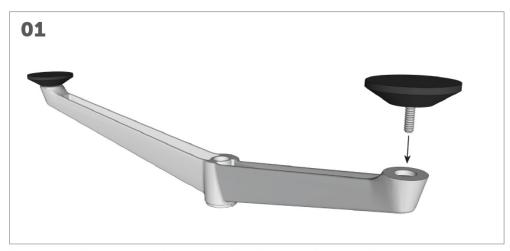
Screw the glides into the base of the fixed feet, leaving the glides one turn from tight (then they can be adjusted easily if the floor is uneven).
