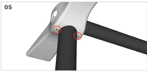
Fully tighten the small screws located at the bottom of each upper wrist to firmly hold the top rail in place.
