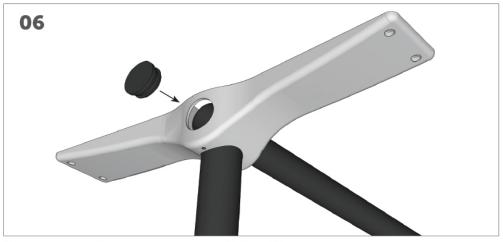
Place the top rail cap into the exposed side of the upper wrist.
