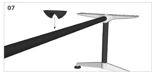
Locate the plastic support bracket over the centre of the top rail, and click into place.
