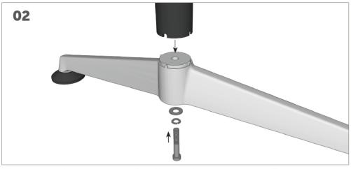
Place the leg tube on top of the fixed foot, making sure each small notch in the bottom of the leg tube is in-line with the bumps on the top of the fixed foot. Fully tighten to maximum tension the large M10x65mm bolts with spring and flat washer.
