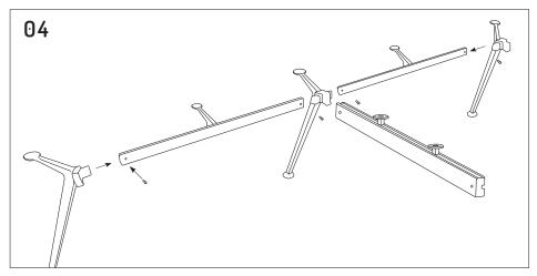
Securely connect legs to rails lengths using the shorter M8x20mm dome head bolts.
