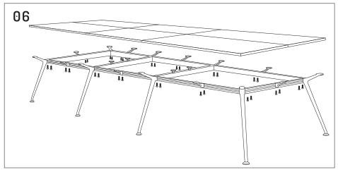
Ensure the work surfaces are centered over the frame. Fully tighten all M5x20mm self tapping screws through each leg rail spacer and support connector bracket into the work surfaces.
