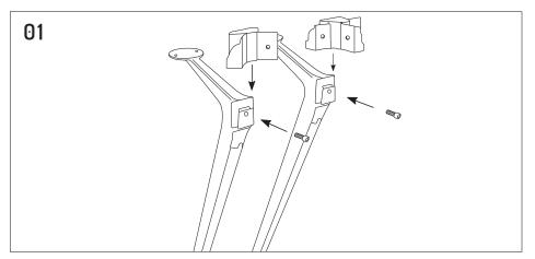
Slide the 2 way and 3 way connectors over each leg, and securely lock into place using M8x20mm cap head bolts.
