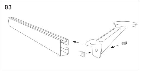
Loosely connect the shorter M8x12mm dome head bolt and slot nut through the metal rail spacer bracket. Slide onto required rails and fully tighten in place.
