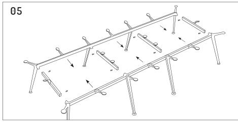
Securely connect legs to rails widths using the shorter M8x12mm dome head bolts.
