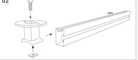
Loosely connect the longer M8x20mm dome head bolt and slot nut through the rail spacer bracket. Slide onto required rails and fully tighten in place.
