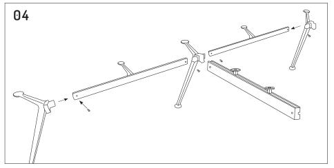
Securely connect legs to rails lengths using the shorter M8x20mm dome head bolts.
