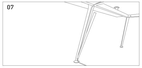
Cancel any power box cable using the magnetic leg cable covers.
