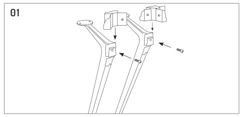
Slide the 2 way and 3 way connectors over each leg, and securely lock into place using M8x20mm cap head bolts.
