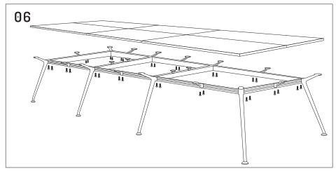
Ensure the work surfaces are centered over the frame. Fully tighten all M5x20mm self tapping screws through each leg rail spacer and support connector bracket into the work surfaces.
