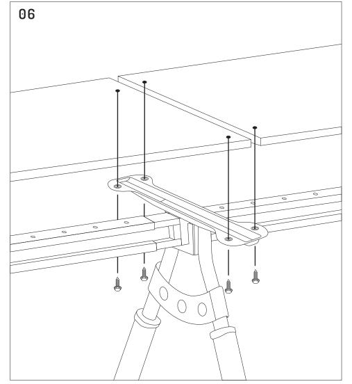
Attach outsider legs + beam to Desk Tops by tightening Scews (O).
