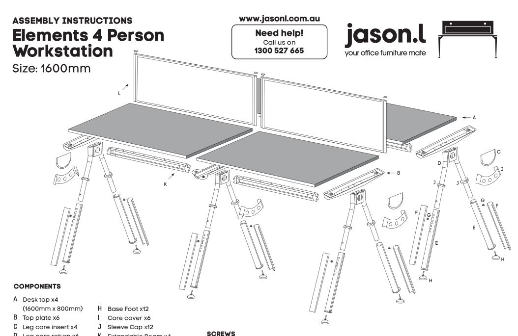
D Leg core return x6 K Extandable Beam x4 E Leg sleeve x12
