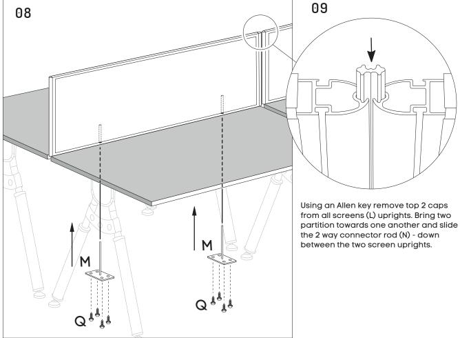
Place 10mm Rod Brackets (M) into designated screen holes. Drill desk tops (A) with H6x30 screws (Q) to assemble the screens.
