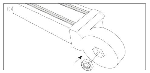
Insert Hex Nut on each Beam Bracket.
