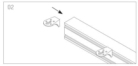
Join 2 L-Bracket through each 1515mm Beam and 1 L-Bracket through each 1150mm Beam.
