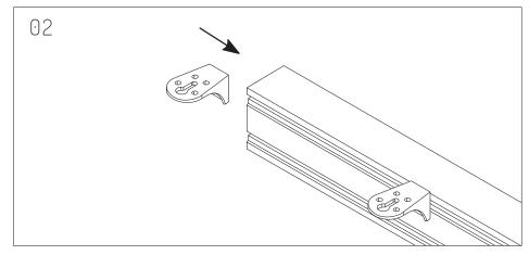
Join 2 L-Bracket through each 1315mm Beam and 1 L-Bracket through each 1150mm Beam.
