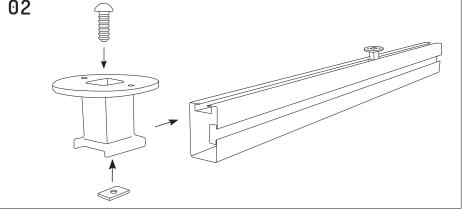
Loosely connect the longer M8x20mm dome head bolt and slot nut through the rail spacer bracket. Slide onto required rails and fully tighten in place.
