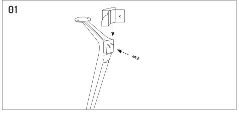
Slide the 2 way connectors over each leg, and securely lock into place using M8x20mm cap head bolts.
