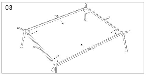
Securely connect legs to rails lenghts using the shorter M8x20mm dome head bolts.
