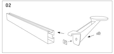
Loosely connect the shorter M8x12mm dome head bolt and slot nut through the metal rail spacer bracket. Slide onto 620mm rails and 1290mm.
