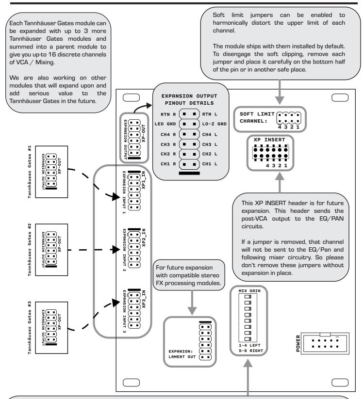
The MIX GAIN switches allow you to further reduce the overall gain of the master output (separate controls for LEFT and RIGHT channels). Below is a diagram that depicts the gain factor reduction. You will usually only need this when using multiple Tannhäuser modules that sum to a very large output.
