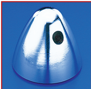
Chrome plated brass prop nuts are great for adding weight to tail heavy aircrafts.
