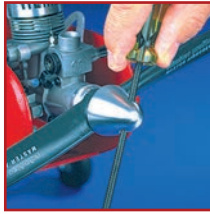
Securely tightens on propeller.
