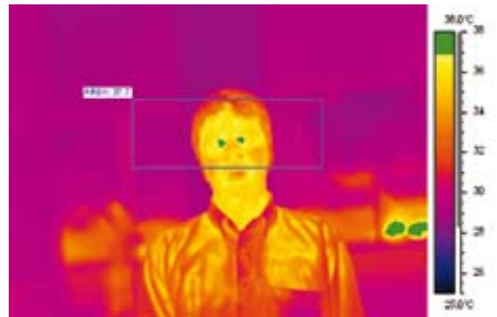
The infrared image clearly shows the hot spots in the corner of the eyes.
