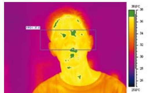
The infrared camera automatically detects the hottest temperature within an area, set by the operator. A color alarm makes it easy to decide whether a person needs further examination or not.
