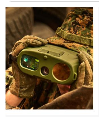
Fully operational at less than 1.6 kilograms, the breakthrough Recon V Ultra Lite provides mid-range target detection, recognition, recording and geo-location with an HD color camera and digitally zoomed multiple FOV thermal channels. Combining a highly accurate laser range finder, GPS, digital magnetic compass and intuitive user interface, targets can be quickly located 24/7.
