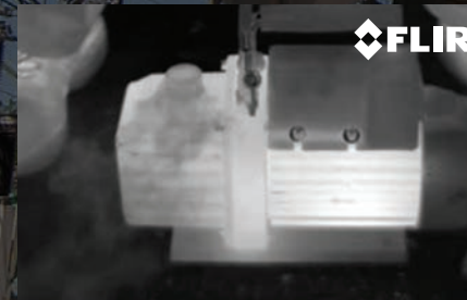
A/C COMPRESSOR - INFRARED IMAGE
