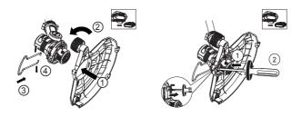
Push the locking knobs and install the auxiliary handle in place.
