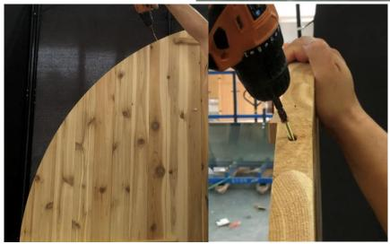
5. Assemble front walls using the same method as the back walls and place the roof middle strip as shown.
